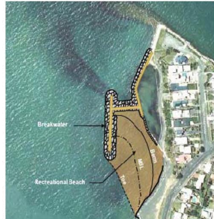
Figure 4.1 H-Shaped Breakwater Layout
