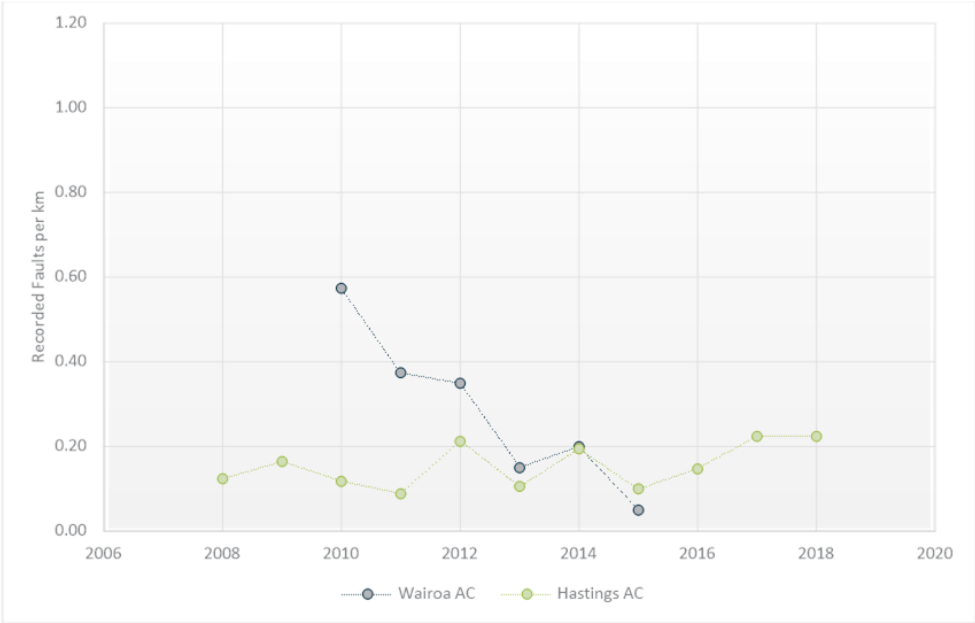
Figure 49 Annual PVC faults normalised by network length
