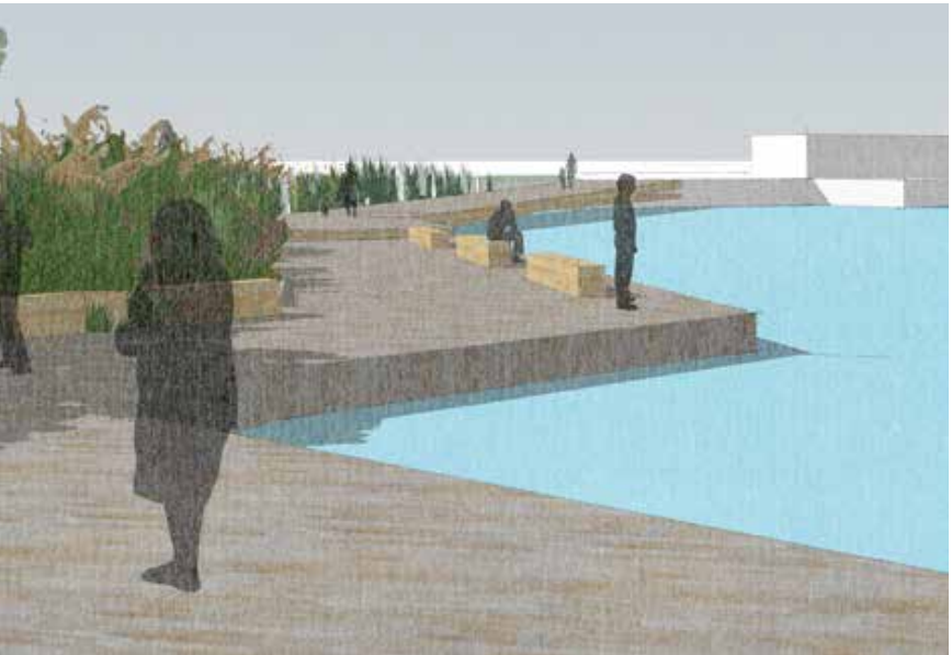
Right. Boardwalk, model boat and fishing deck across end of inner harbour from West Quay to Sailing Club Reserve. Hardwood timber deck, incorporating steps and seating elements. Estuarine and brackish planting extending from recontoured waters edge.
