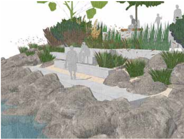
Left & Above. Large scale concrete seating elements at key locations accessed from the widened upper boardwalk create off-line spaces to sit and watch the activity of the channel. Interplant upper areas of revetment with native grass and groundcover species.
