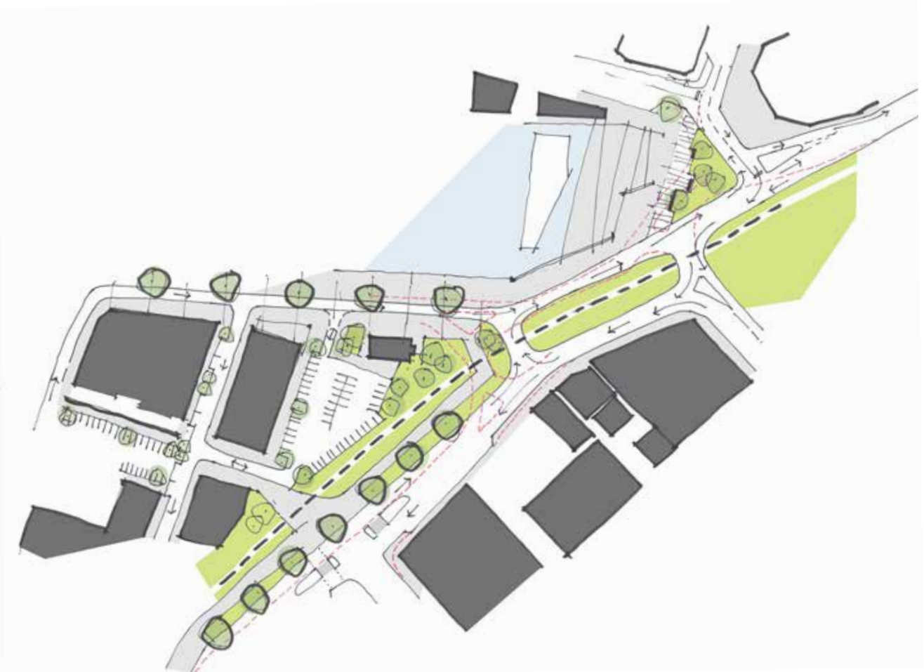
One-way Customs Quay (east bound), enableline a reduction in length of the 'peanut' roundabout. Simplification of kerb alignment approaching Coronation Street. Planted island incorporated into footpath space at end of Iron Pot.
