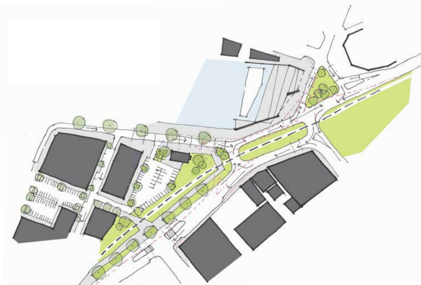
One-way Customs Quay (east bound), enableline a reduction in length of the 'peanut' roundabout. Simplification of kerb alignment approaching Coronation Street, including amalgamation of splitter islands at end of Iron Pot to created large planted island.
