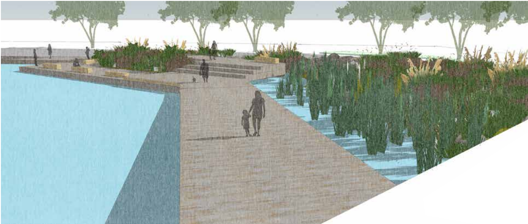
Right. Boardwalk, model boat and fishing deck across end of inner harbour from West Quay to Sailing Club Reserve. Hardwood timber deck, incorporating steps and seating elements. Estuarine and brackish planting extending from recontoured waters edge.
