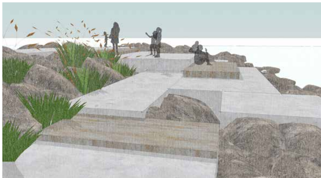
Above. Concrete, limestone and timber headland extends out from point, enabling easier access and providing opportunities for seating and location for fishing.
