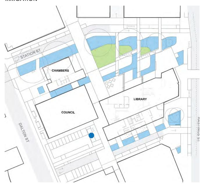
A 'water sensitive design' approach will be taken to cleanse stormwater through planted 'raingardens' that remove pollutants before entering the wider system.
