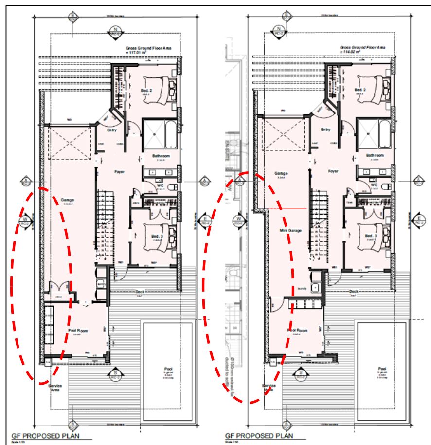
Figure 5: Amended floor plan demonstrating the extent of the dwelling to be setback 1.0m from the boundary in comparison to the floor plan of the adjacent dwelling.
