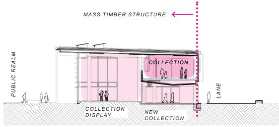
Fig 49. Cross section through the library's collection display area (looking east) with the Public Realm to the left of the building and the southern Lane to the right.
