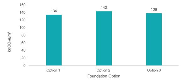
Figure 3: Upfront Carbon of foundations for each option
