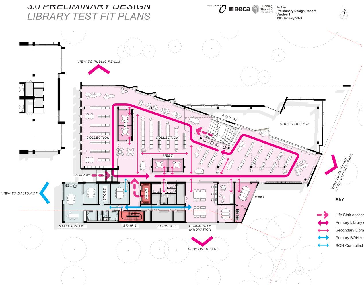
Fig 64. Level 1 Test Fit Plan indicating stair access, room access, circulation and indicative shelving/ furniture arrangement.
