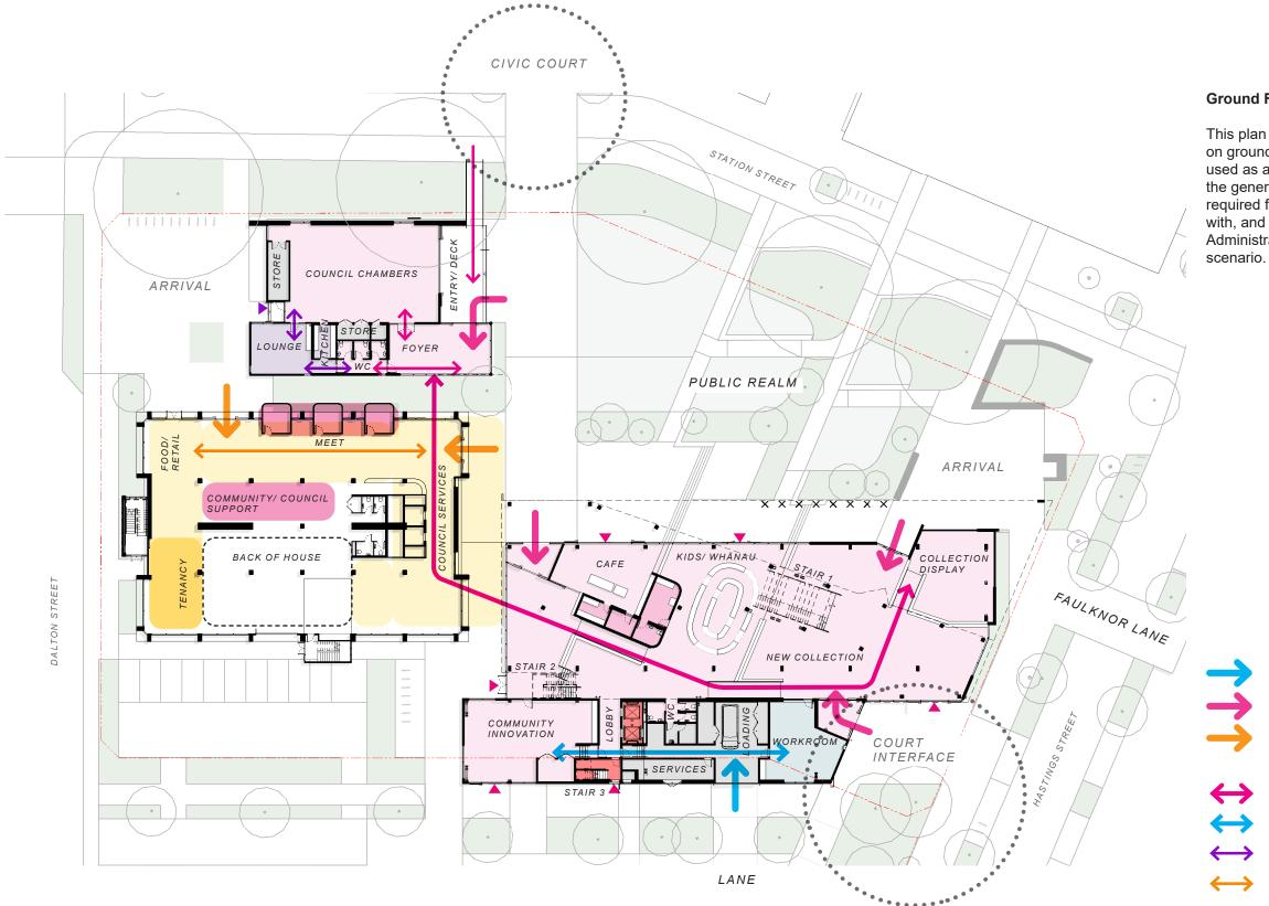
Fig 42. Ground Floor Plan - This plan shows the distribution of the programme on the ground floor when the Chambers is being used as a Community Room by the general public and / or the library. Note the CAB (existing Library Tower) is out of scope. Indicative future design shown.
