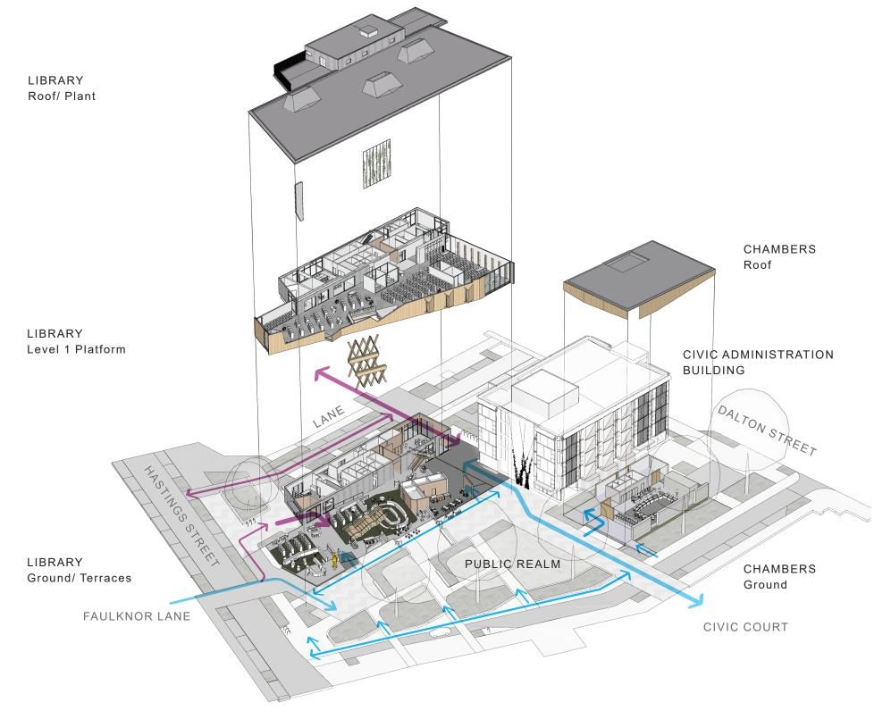
Fig 40. Exploded Axonometric of the Library, Civic Chambers and Public Realm. Note the CAB (existing Library Tower) is out of scope. Indicative future design shown.
