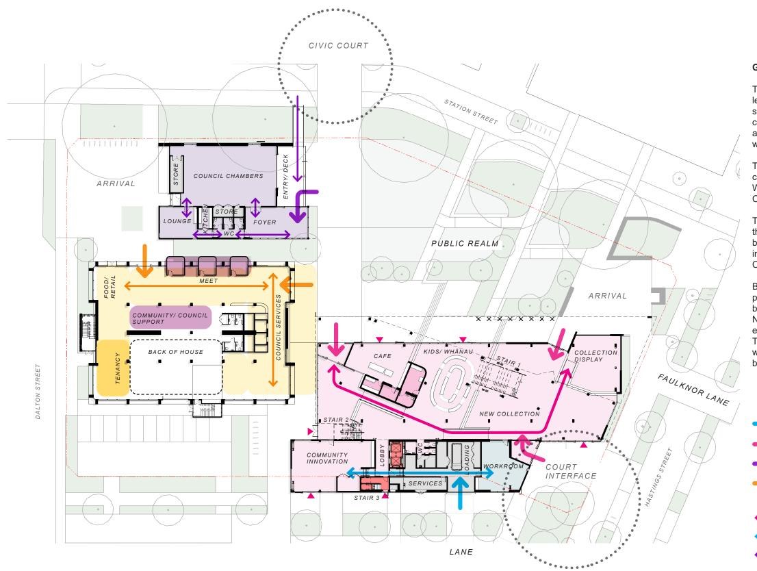
Fig 41. Ground Floor Plan - This plan shows the distribution of the programme on the ground floor when the Chambers is being used by Council. The anticipated interface with, and integration of, the ground floor of Civic Administration Building is also indicated. Note the CAB (existing Library Tower) is out of scope. Indicative future design shown.
