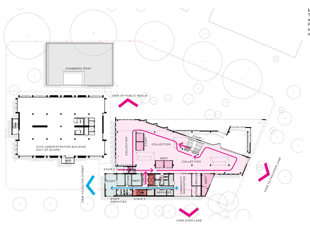
Fig 43. Level 1 Plan - This plan shows the distribution of the programme on the first floor, where most of the collection will be housed. Note the CAB (existing Library Tower) is out of scope. Indicative future design shown.
