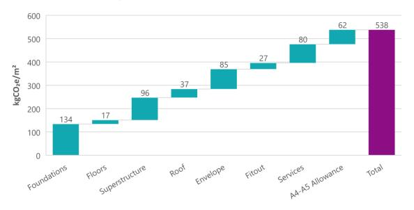
Figure 2: Upfront carbon breakdown by element
