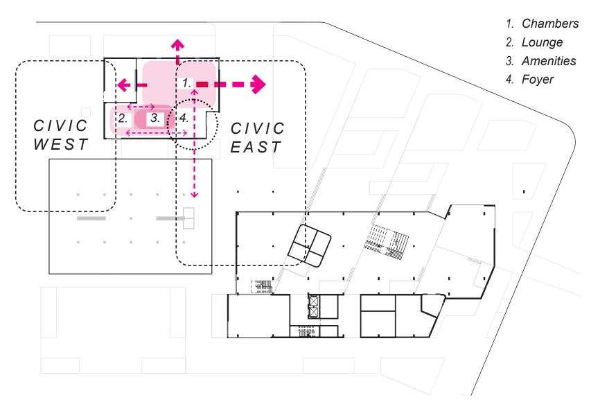
Fig 71. Plan diagram of the of proposed Chambers building, highlighting key interfaces with the Public Realm and Civic Administration Building.
