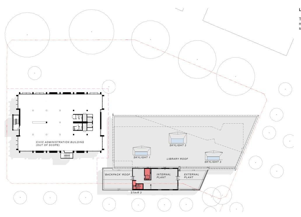
Fig 44. Level 2 Plan - This plan indicates the internal plant and external plant areas as well as the three skylights providing natural light to deeper parts of the level 1 collection space. Note the CAB (existing Library Tower) is out of scope. Indicative future design shown.
