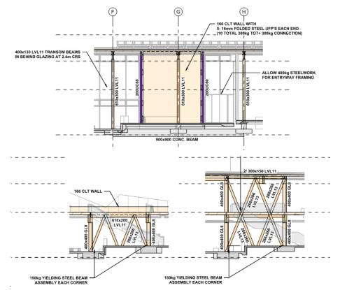
Figure 2.4 – Timber Bracing Elements
