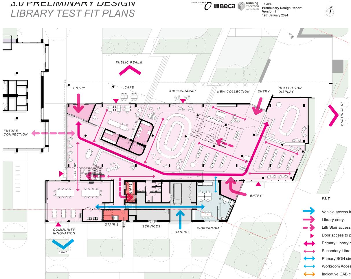
Fig 63. Ground Floor Test Fit Plan indicating building entries, room access, circulation and indicative shelving/ furniture arrangement
