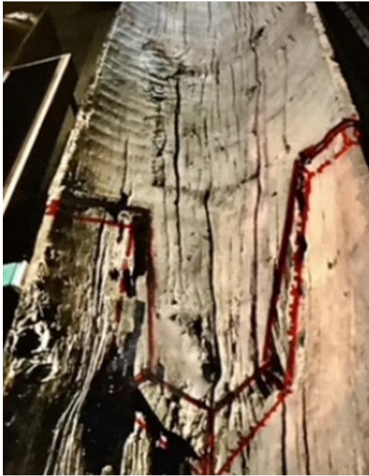
Fig 1: Haumi joint in historical waka construction
