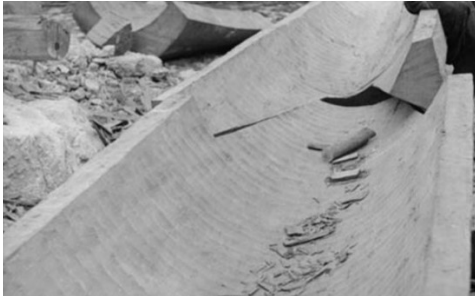
Fig 1.6.2 Haumi joint under construction
