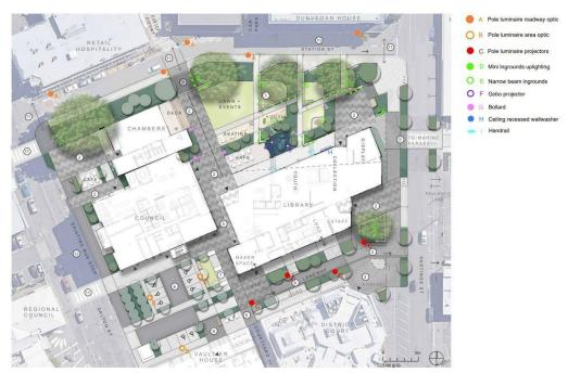
Figure 2: Lighting Concept Plan for the Library, prepared by Energy Light
