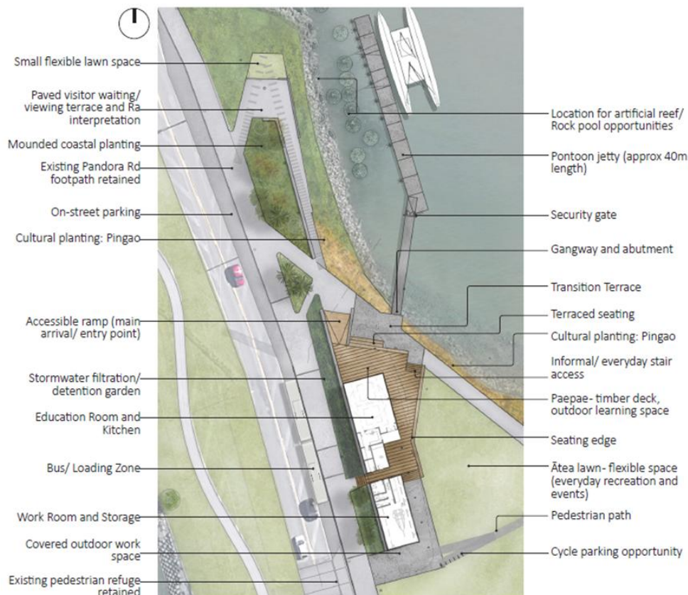
Plan showing spatial arrangement of features and spaces within the Waka Hub, and how they relate to each other.
