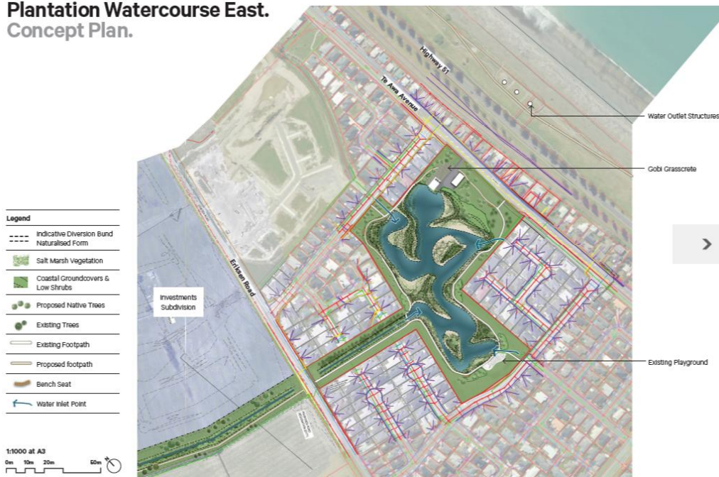
Figure 2: Serpentine Pond reserve at Te Awa Avenue drainage concept plan.
